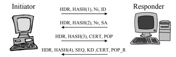
To construct the first GDOI message the initiator chooses Ni and creates a nonce payload, builds an identity payload including the group identifier, and generates HASH(1).
