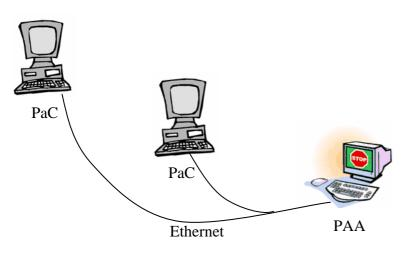
When using a shared medium like ethernet, the link between PaC and PAA is assumed to be not physical secure.
